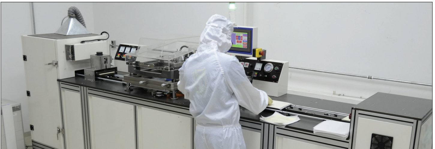
Screen Printing of Electrodes and Stacking of Ceramic Layers
