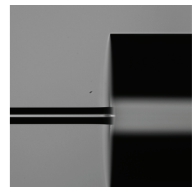
Ø1.25 mm Silica End Cap Fused onto Ø125 µm Fiber
